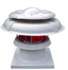
Fiberglass Upblast Roof Exhauster - Direct Drive Sizes 12" through 18" (30cm through 45cm) Capacities from 500 to 3,400 CFM (14 to 96 m3/min)
