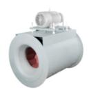
Fiberglass In-Line Centrifugal fan combines the design advantages of the axial flow fan with the performance characteristics of the centrifugal fan. These compact inline fans are the ideal selection for indoor clean air applications including intake, exhaust, return, or makeup air systems where space is a prime consideration. Available in belt drive or direct drive, square or tubular.
